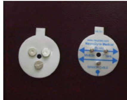
1. AE-131 circular surface EMG disposable electrode
