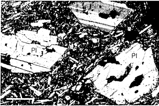
Fig. 11. Photomicrograph of basalt xenolith in Byeoldobong tuff. Pl, plagioclase (XPL, scale bar: 0.5 mm).
