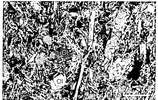
Fig. 8. Photomicrograph of Shinheungri basalt. Ol, olivine; Py, clinopyroxene; Pl, plagioclase (XPL, scale bar: 0.5mm).
