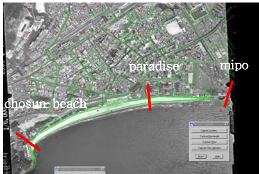
FIGURE 15. Base line arrangement for seashore width measurement
