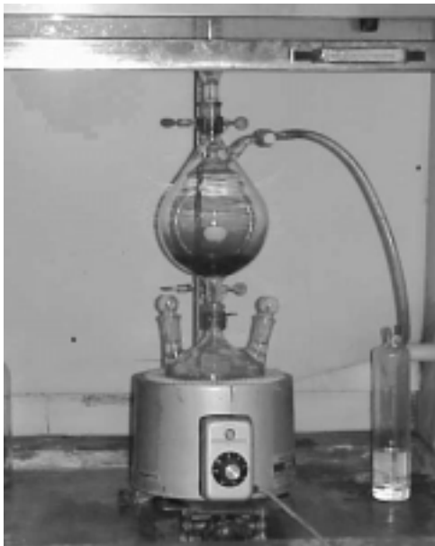
Fig. 1. The intercalation process of \text{SO}_3 into flake graphite.
