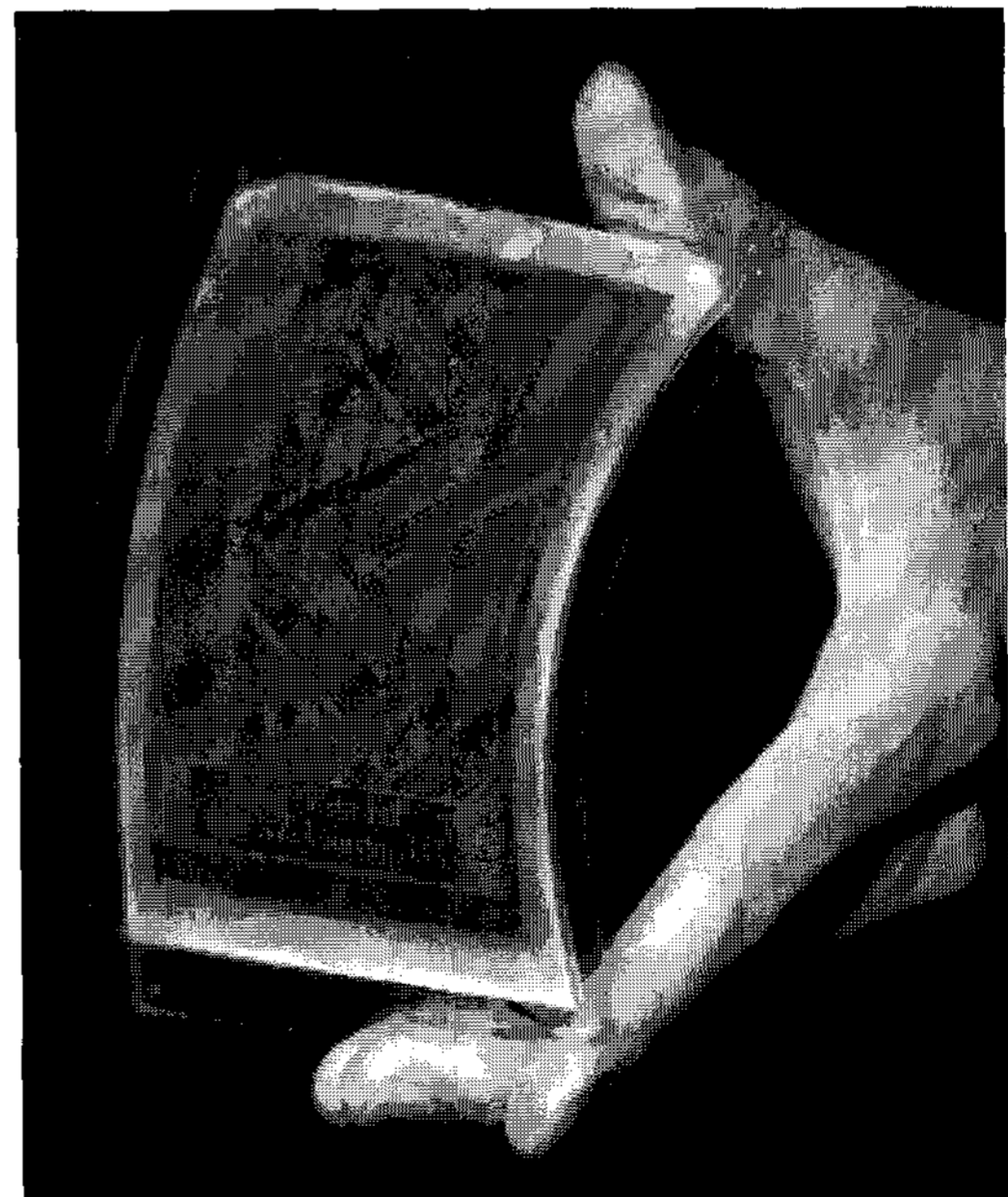
Fig. 1. A four inch square, 320 by 320 pixel bistable cholesteric display made using flexible polyester substrates.
