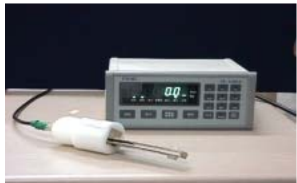
Fig. 2. A photograph for a primary model of the measuring device for bite force
