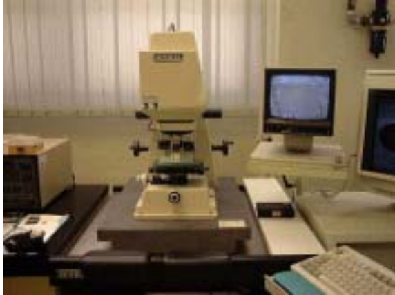
Fig. 6. Three-dimensional Imaging surface structure analyzing system (NT-2000).
