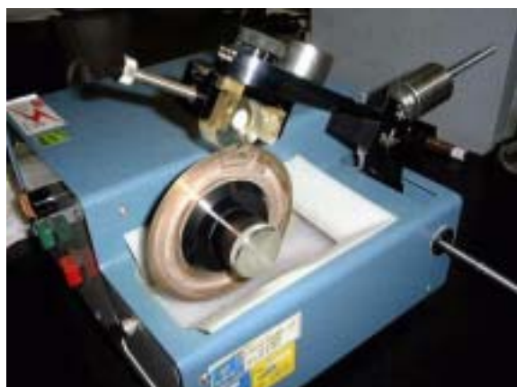
Fig. 2. Teeth samples were cut flat by occlusal or buccal or lingual reduction with a slowly rotating diamond blade under running water.
