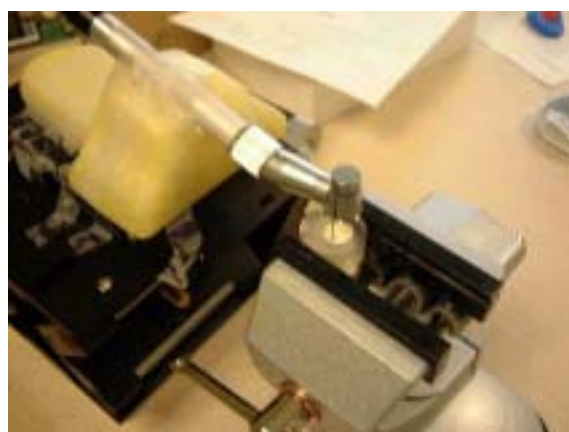
Fig. 5. Focal length(9 mm) was precisely reproduced using the guide pin attached on the side of handpiece.
