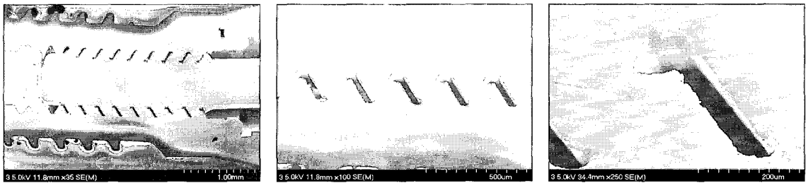
Fig. 6. Pictures of implant-teflon coated titanium alloy screw assembly in Steri-Oss implant system in SEM (Magnification \times 35 , \times 100 , \times 250 ).
