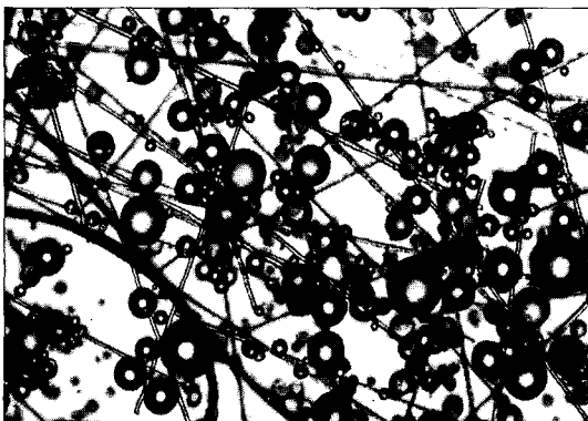
Fig. 12. Mixture of PMMA powder and glass fibers. Transmitted light. Original magnification \times 20 .
