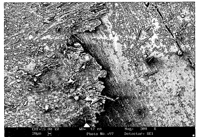
Fig. 10 (b) Damaged carbon tube of C30-3T
