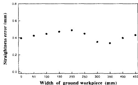
Fig. 19 Straightness error of a ground workpiece
