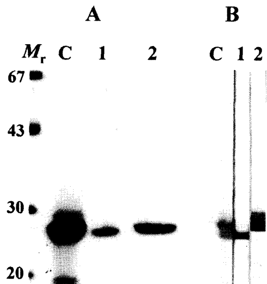
Fig. 1. (A) SDS-PAGE analysis of the purified 28 and 27 kDa cysteine proteases of P. westermani metacercarial ESP. M_r , molecular mass markers in kDa; C, crude ESP; 1, 27 kDa cysteine protease eluted through flow-through fraction; 2, 28 kDa cysteine protease purified in 0.2 M salt concentration. (B) Reactivity of anti-27 and anti-28 kDa cysteine proteases of metacercarial ESP analyzed by immunoblotting. Lanes 1 and 2 denote the reactions with anti-27 and anti-28 kDa antibody, respectively. Other markings are same as in (A).
