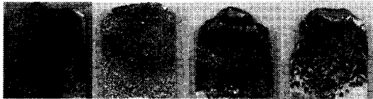
(a) T=585°C (b) T=595°C (c) T=615°C (d) T=680°C Fig. 5 Foamed aluminums at various temperatures of molten Aluminium (N = 1700rpm, V h = 20°C/min, T = T f )
