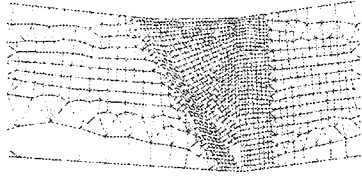
Fig. 6 Two dimensional finite element model for the multipass weld
