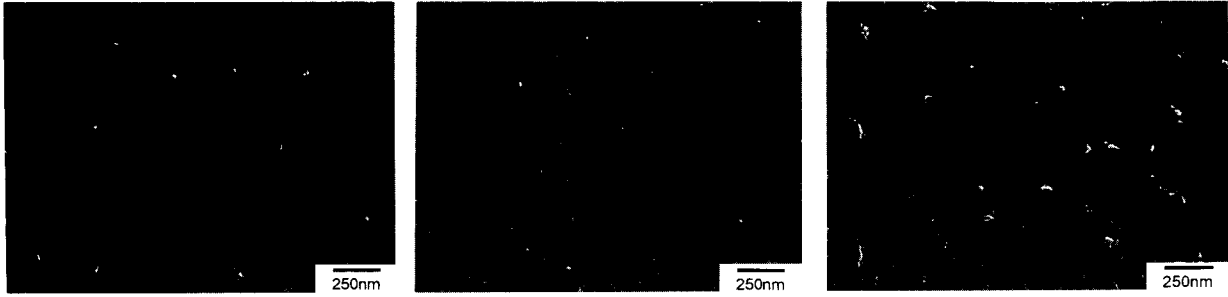
Fig. 12. SEM microstructures of (a) conventional PECVD (b) mesh-type PECVD (c) 300°C, 20W, DC bias : 200V, H 2 : 37.5sccm specimen (91% overlapping : scanning mode, 340mJ/cm 2 )
