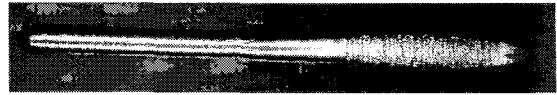
Fig. 7 Example of a micro carbon rod with varying surface quality ( E = 2.8W , p = 760Torr )
