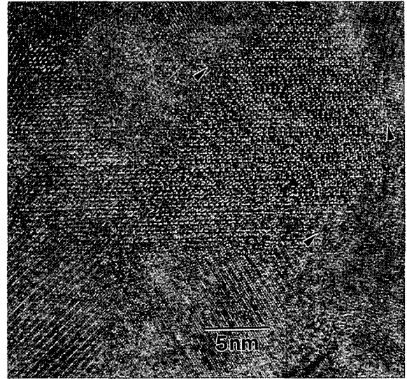
Fig. 5. High resolution micrograph of nanocrystalline Nd_4(Fe_{0.85}Co_{0.15})_{82}B_{10}Mo_3Cu alloy.
