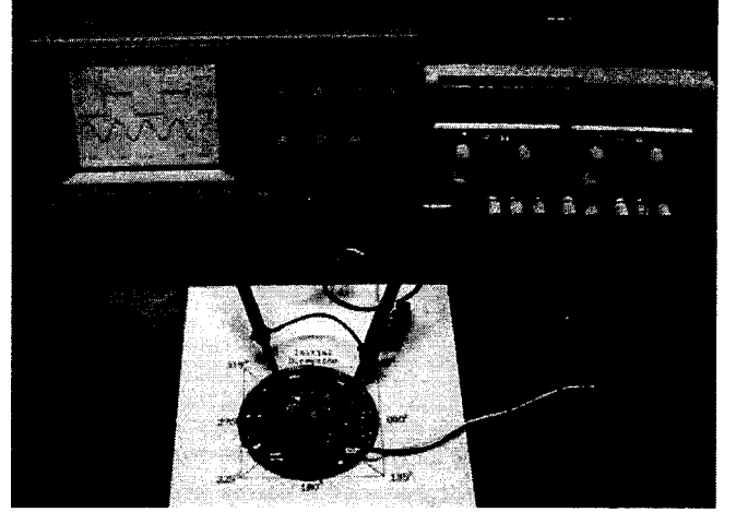
Fig. 9 Test environment set-up in a normal room. Realized Flux-gate compass circuitry (below front), Oscilloscope with 100MHz resolution (top left), and Power supply (top right).
