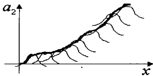
Fig. 5 Output of the RBF network as a local response
