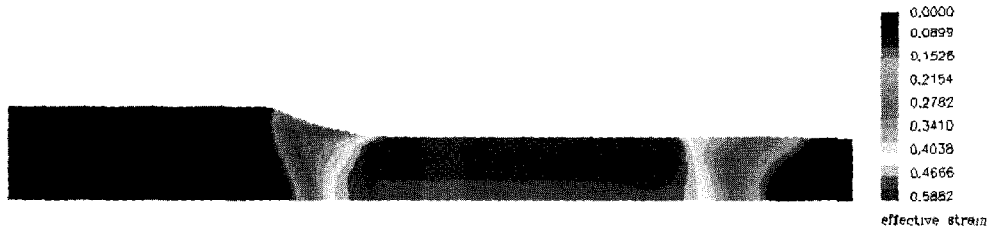
Fig. 5 Distribution of effective strain with rigid-plastic FE simulation
