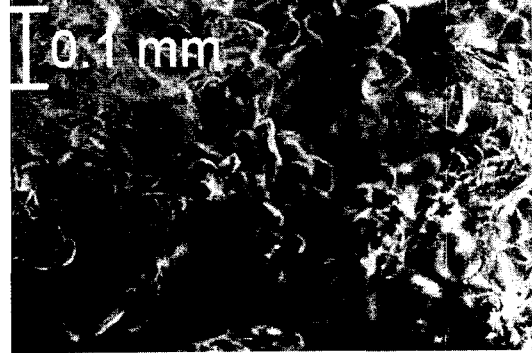
Fig. 4 Snapshot of ice slurry (EG 4 vol%).
