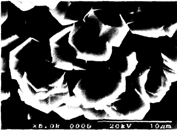
Fig. 6. SEM micrograph of Ni substrate bias-treated for 10 mins and then deposited for 2 hrs without bias with 2 vol% \text{CH}_4 at 925^\circ\text{C} .
