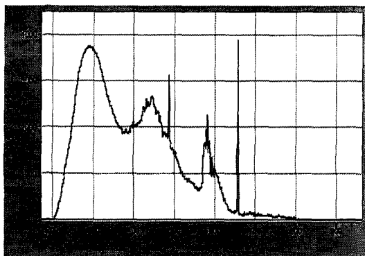
Fig. 1. The spectrum of the UV light source.
