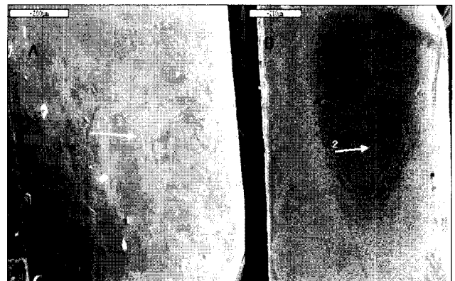
Fig. 10. One-Up Bond F의 Smearing시 SEM A: fractured dental surface, B: fractured resin surface. 1: bonding agent, 2: resin
