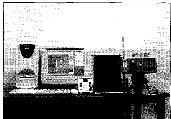
Fig. 1. Infrared thermal imaging system.
