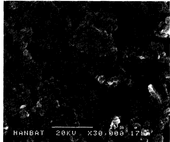
Fig. 2. SEM micrograph of particle shape of ZnS:Cu (0.03 M) nano-crystals.
