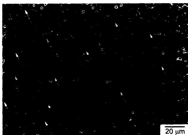
Fig. 1. The microstructure of the specimen sintered at 1550°C for 4 h.
