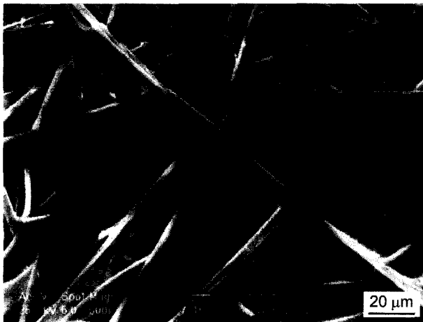
Fig. 1. SEM image of ceramic paper before impregnation adsorbents.
