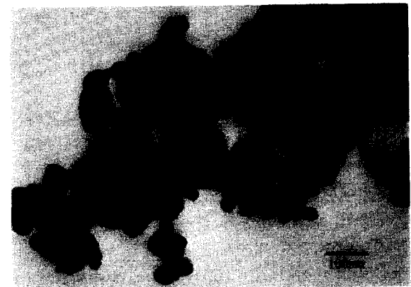
Fig. 5. TEM diffraction patterns and micrographs of the PCFN powders calcined at 700°C.
