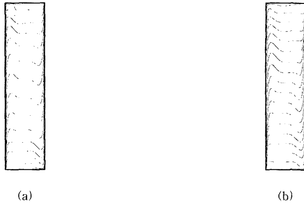
Fig.2 Isotherms predicted by the two-layer model with AFM (a), and by the \overline{v-v-f} model with AFM. (b)
