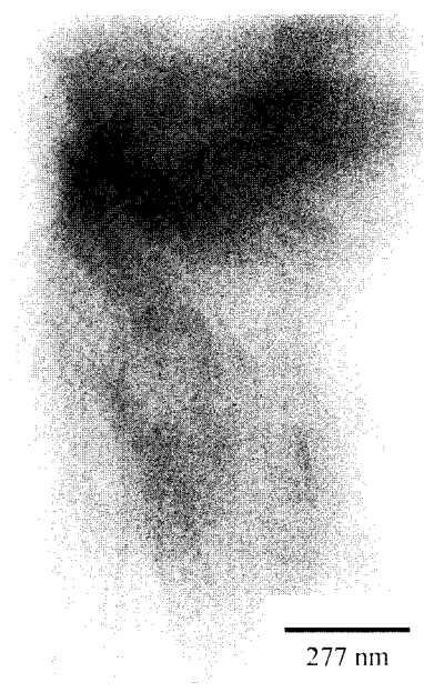
Figure 2. Transmission electron microscopic photograph of nanocomposite containing 2 wt% 12Me-MMT in EVA-12 matrix.
