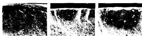
Fig. 20 SEM photographs of fracture surface around crack initiation point for specimen SUP 7 under 2 stage shot-peened
