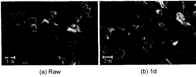
Fig. 11. SEM photographs for C 3 A · CaCl 2 · 10H 2 O-CaCl 2 system.
