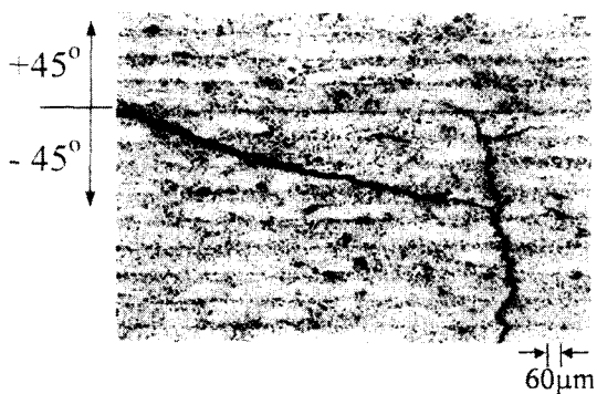
Fig. 9 Microscopic photograph of the cross-section near the free edge of a [+45_6/-45_6]_s laminate. Several transverse cracks and delaminations are revealed
