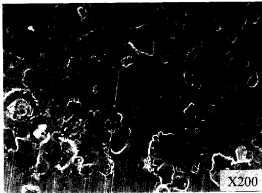
(a) Corrosion surface
