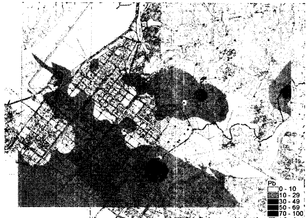
Fig. 9. Distribution of Pb contents of soils in the vicinity of Shi-Hwa industrial complex region (Unit: mg/kg).
