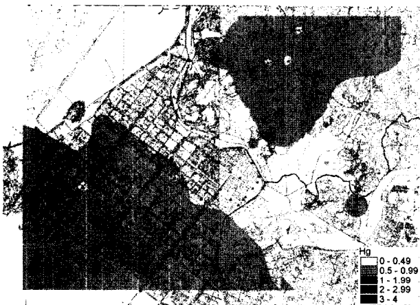
Fig. 7. Distribution of Hg contents of soils in the vicinity of Shi-Hwa industrial complex region (Unit: mg/kg).
