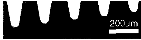
Fig. 7 Micrograph of a mold (Spindle revolution speed: 27,500rpm, Feed rate: 0.6mm/sec, Depth of groove: 150mm)
