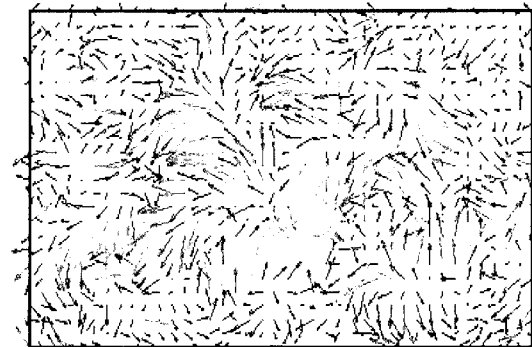
Fig. 18 Instantaneous velocity vector distribution along the test tube for Re = 2,724 after removing error vectors.
