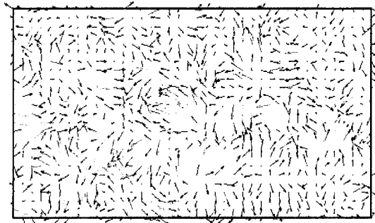
Fig. 17 Instantaneous velocity vector distribution along the test tube for Re = 2,500 after removing error vectors.
