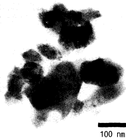
Fig. 1. A transmission electron micrograph showing the UO_2 particles.
