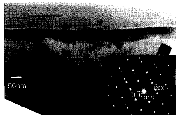
Fig. 4. XTEM and SADP of the sample deposited at 650°C for 15 min along the <011> zone axis.
