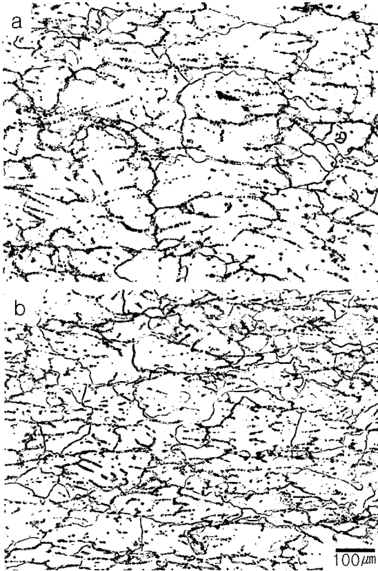
Fig. 8. Optical micrographs of as-forged Al 6061-T6 continuous cast bar forged with either (a) crank press or (b) hammer press, respectively.
