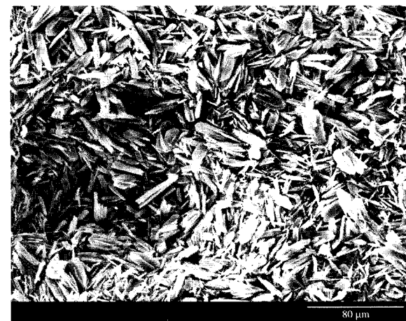
Fig. 2. Scanning electron micrograph of the powder precipitate collected along with the substrate treated with the solution A of pH 6.7 by the thermal dissociation method.
