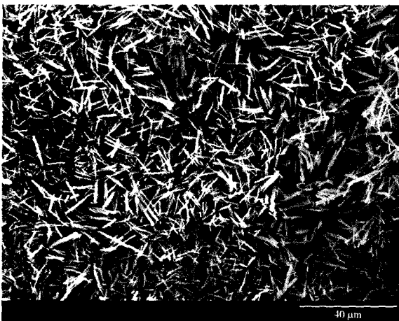
Fig. 4. Scanning electron micrograph of the powder precipitate collected along with the substrate treated with the solution A of pH 10.6 by the thermal dissociation method.
