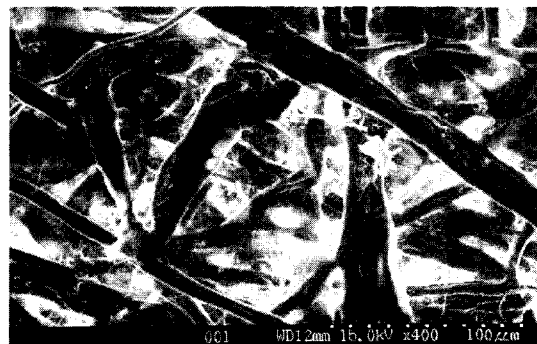
Fig. 5. Scanning electron micrograph ( \times 400 ) of the surface of a handsheet prepared with the separated refining of staple and linter fiber stocks.
