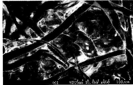
Fig. 2. Scanning electron micrograph ( \times 450 ) of the surface of a handsheet prepared with the mixed stock of staple and linter at a rate of 50 to 50 percent after refining up to 50oSR.
