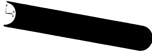
Fig. 2. Meshes of a local wall thinned pipe
