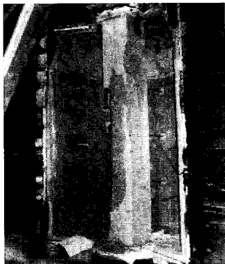
Fig. 3 Furnace and a fire damaged column after 60 minutes of heating
