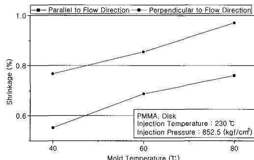
(b) PMMA and disk specimen
