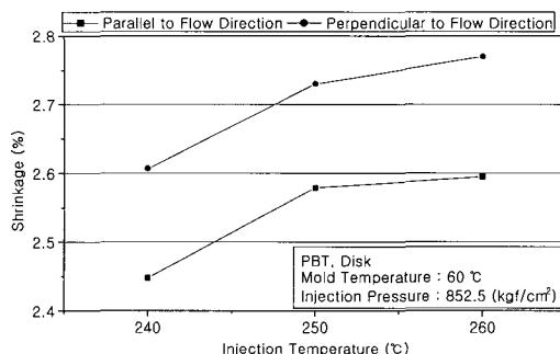
(c) PBT and disk specimen
