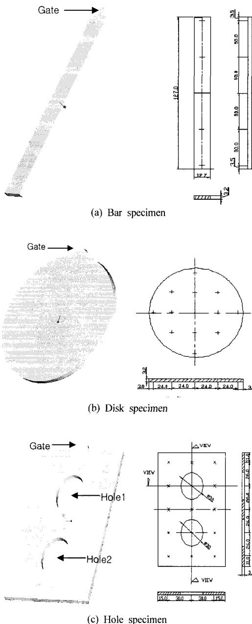
Figure 1. Shapes of specimens and location of gate for injection molding.
