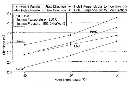
(b) PBT and hole specimen
