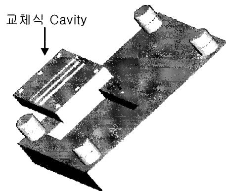
Figure 2. Schematic drawing of cassette mold for the injection molding of test specimens.
