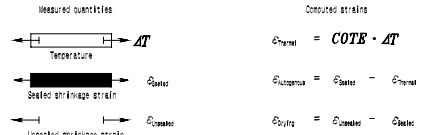
Fig. 10 The procedure for computing the corresponding thermal, autogenous, and drying shrinkage components
