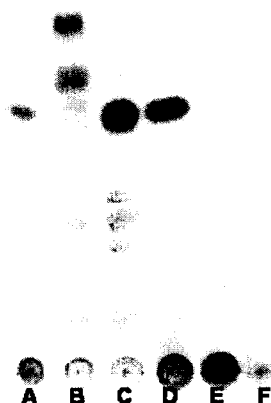
Fig. 1. TLC analysis of scutellaria barbata solvent extracts. A, methyl alcohol extract; B, hexane extract; C, methyl chloride extract; D, ethyl acetate extract; E, buthanol extract; F, water extract.
