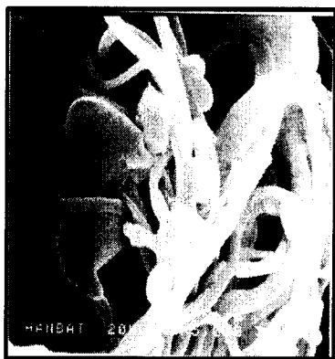
a) \times 5,000 : low molecule weight polyethylene wax
