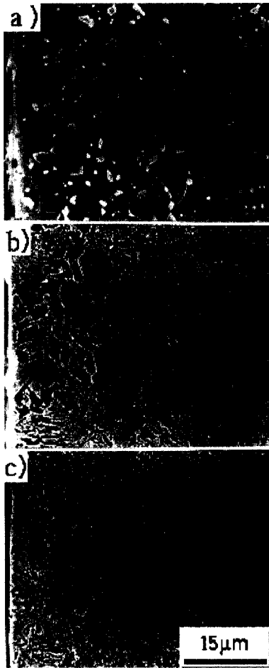
Fig. 1. Cross section SEM micrographs of the tongue materials (a; base metal, b; quenching & tempering, c; carbon restoration quenching & tempering).
